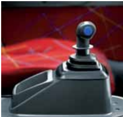
The EuroTronic gearbox can operate completely automatically by simply pressing a button on the left of the lever. In this configuration it is the electronic control unit that governs gear changing.
