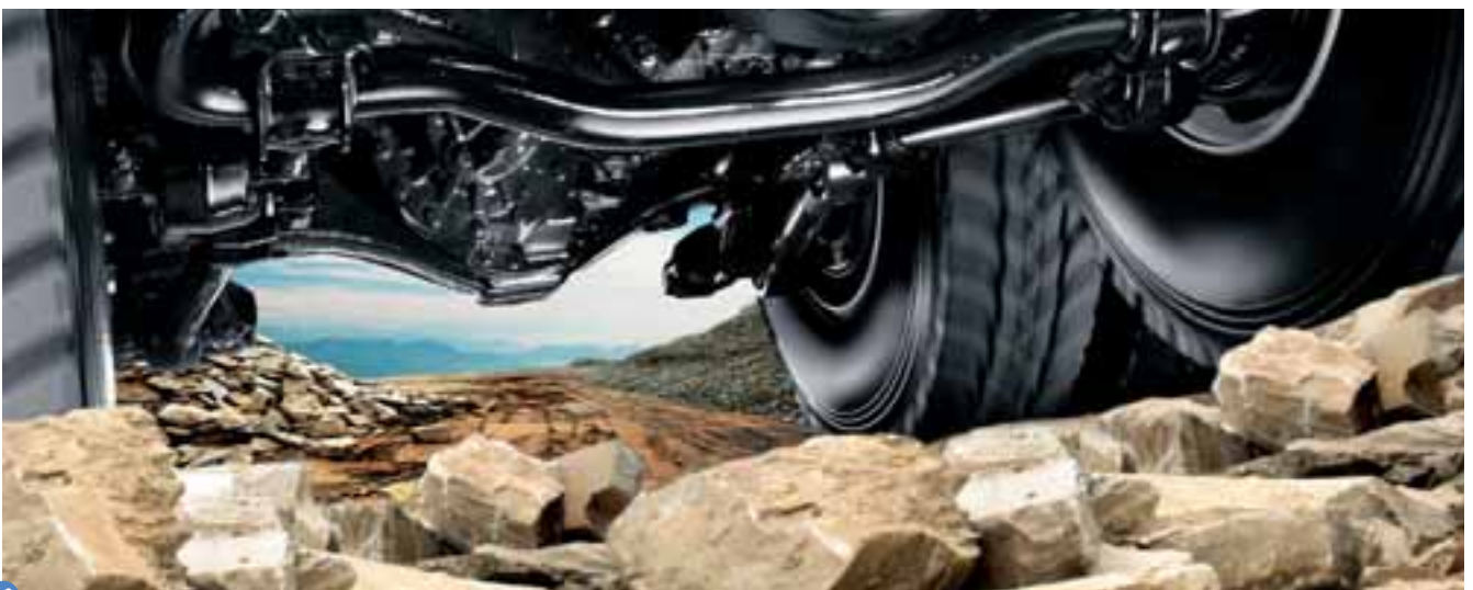
High ground clearance thanks to double reduction axles.
